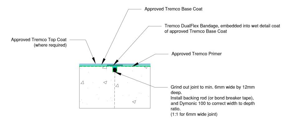
Consult Tremco for project specific advice for cracks/ joints with significant movement anticipated.
